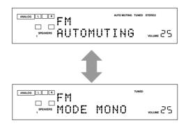
AUTOMUTING: When a program is broadcasted in stereo, you will hear stereo sound; when in monaural, you will hear monaural sounds. This mode is also useful to suppress static noise between stations. The AUTO MUTING indicator lights up on the display.
